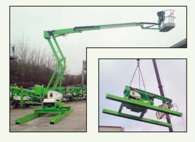
Lifting points allow the **DR15** to be craned into position quickly and easily and the base frame 'sled' has a variable width facility to cater for differing pitches of profiled steelwork. A 1.80m wide cage provides more room for materials and tools and a 150° fly-boom with 100° cage rotation, helps to increase accuracy when positioning.
